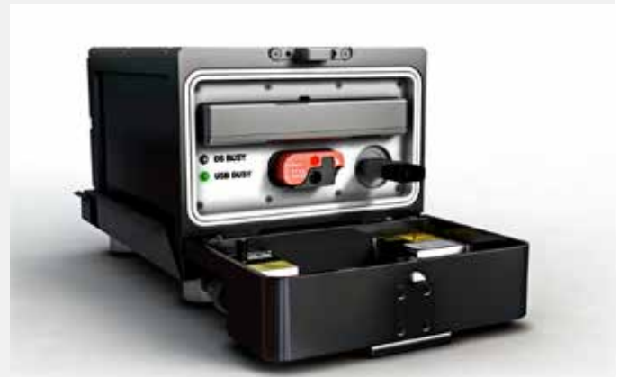
SDR WITH ACCESS PANEL OPEN, REVEALING THE KSU AND SDS
