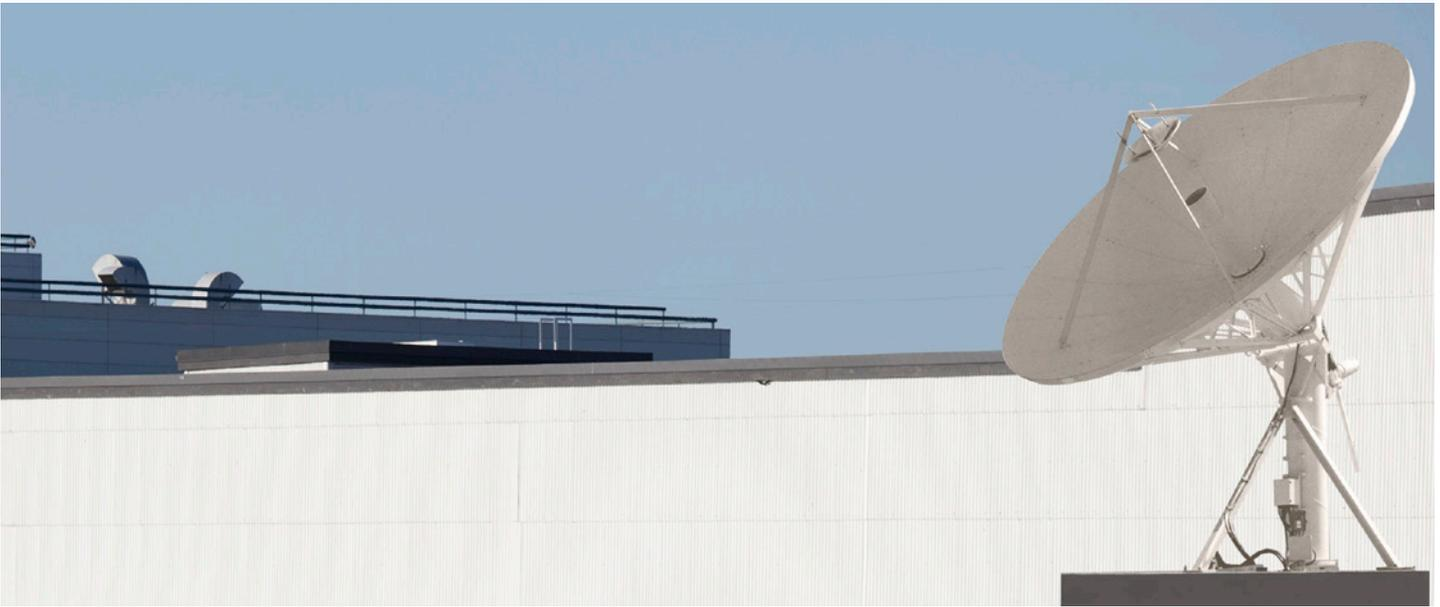
Model 8010D is a 7.3 meter earth station antenna that provides high gain and excellent pattern characteristics through the use of precision stretch-formed reflector panels and advanced computer-shaped Gregorian optics.
