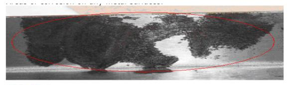
**Caution:** Small areas of rust are acceptable where plating is removed by a standard manufacturing or welding process, e.g. sheared (cut) edges.
