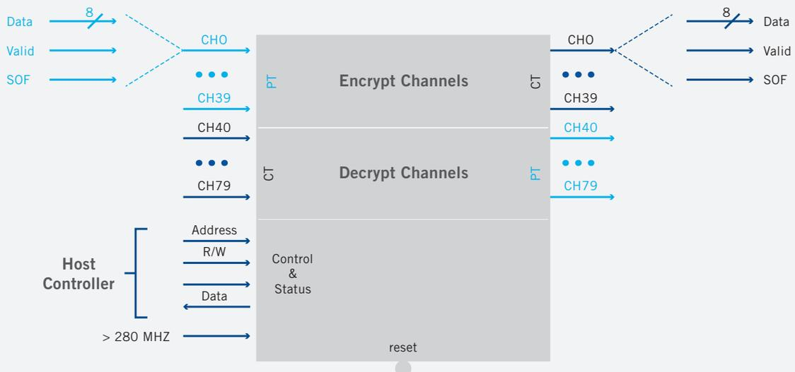
Viasat’s security core interfaces to the host system through multiple independent encrypt/decrypt data channels and a simple control and status bus. All interfaces are synchronous to the 280 MHz clock.
