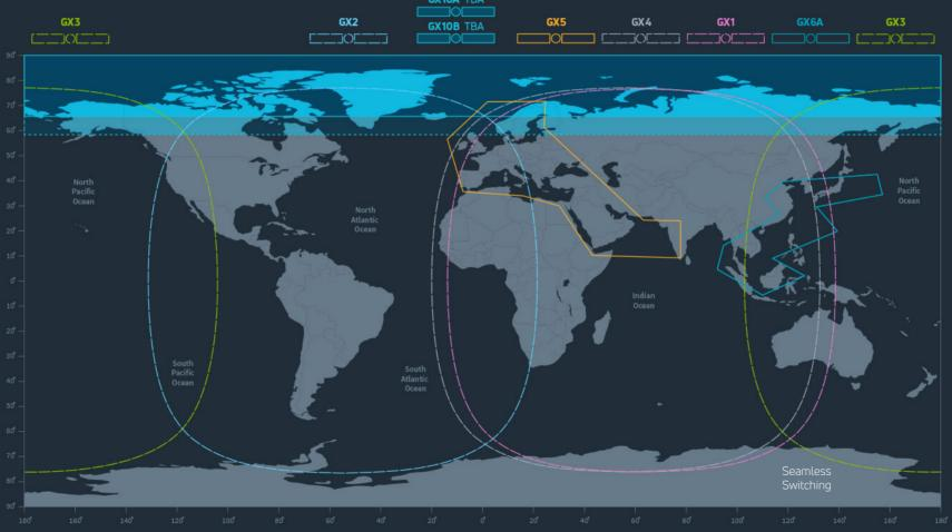
Each payload has two steerable beams interoperable with Mil-Ka networks for government use above 57° North.
