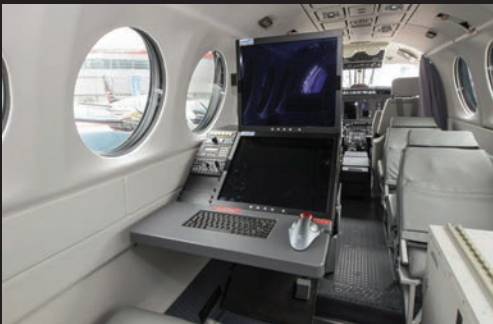
This modular mission management console is part of a bespoke King Air Solution.
