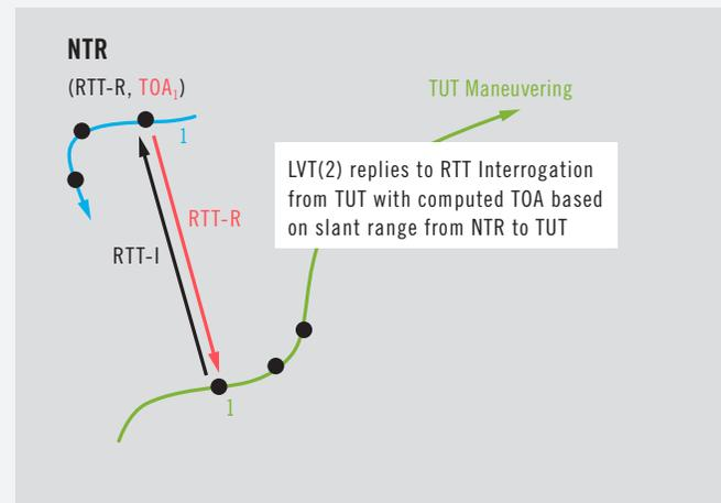
These delays simulate the propagation delay due to the slant range between the transmitter's position and the receiver's position and allow the receiver to make precise time-of-arrival measurements.
