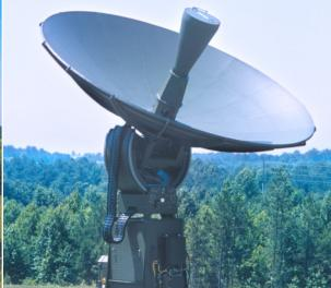
The mobilizer concept is totally self-contained and provides a stable operating platform when fully deployed. The reflector uses a quick-latching mechanism to permit rapid assembly and disassembly of the reflector. These panels are then stored within racks on the trailer deck during transport. Designed for transport by a C-130 or similar aircraft, the system also meets all specifications for road transport.
