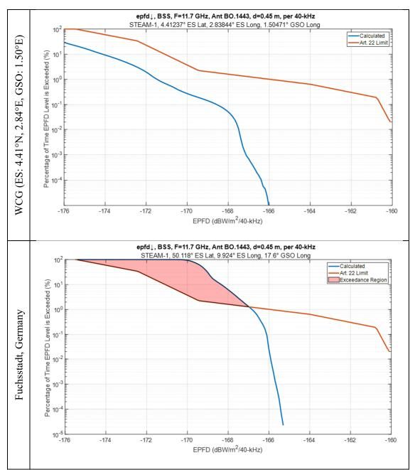
Figure 3 - Comparison of STEAM-1 EPFD↓ at 11.7 GHz with 0.45 cm GSO ES for WCG and for Fuchsstadt, Germany (50.118°N. 9.924°E) with GSO Satellite at 17.6°E
