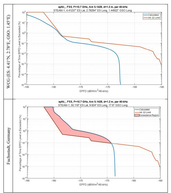
Figure 1 - Comparison of STEAM-1 EPFD↓ at 10.7 GHz with 1.2 m GSO ES for WCG and for Fuchsstadt, Germany (50.118°N. 9.924°E) with GSO Satellite at 17.6°E
