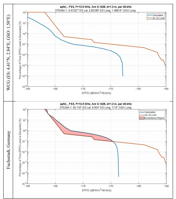
Figure 8 - Comparison of STEAM-1 EPFD↓ at 12.5 GHz with 1.2 m GSO ES for WCG and for Fuchsstadt, Germany (50.118°N. 9.924°E) with GSO Satellite at 17.6°E
