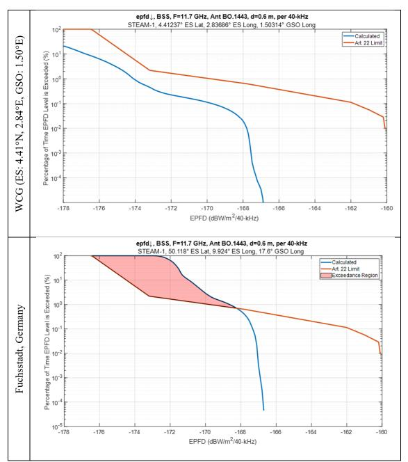
*Figure 4 - Comparison of STEAM-1 EPFD↓ at 11.7 GHz with 0.6 m GSO ES for WCG and for Fuchsstadt, Germany (50.118°N. 9.924°E) with GSO Satellite at 17.6°E*
