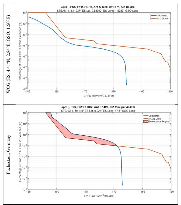
*Figure 2 - Comparison of STEAM-1 EPFD↓ at 11.7 GHz with 1.2 m GSO ES for WCG and for Fuchsstadt, Germany (50.118°N. 9.924°E) with GSO Satellite at 17.6°E*
