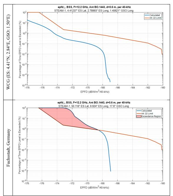
*Figure 7 - Comparison of STEAM-1 EPFD↓ at 12.2 GHz with 0.6 m GSO ES for WCG and for Fuchsstadt, Germany (50.118°N. 9.924°E) with GSO Satellite at 17.6°E*
