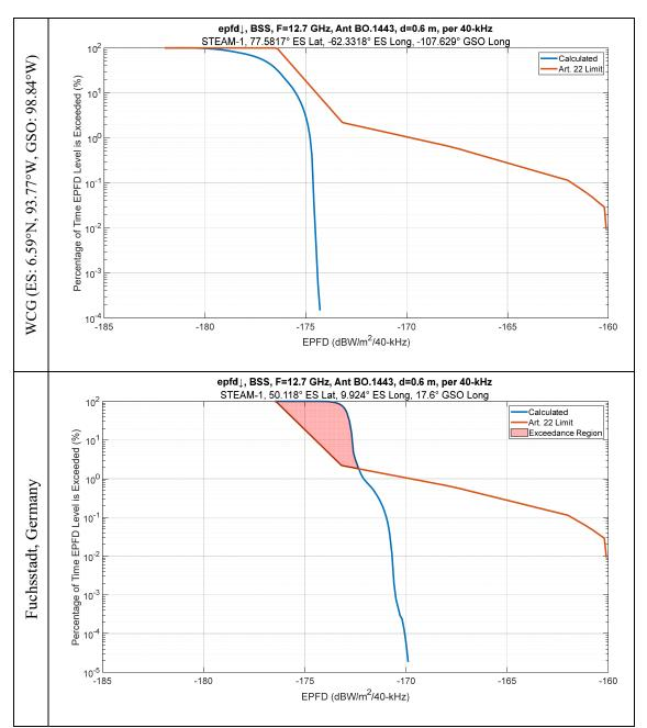
Figure 18 – Comparison of STEAM-1 (ID 121520025) EPFD  $\checkmark$  at 12.7 GHz with 0.6 m GSO ES for WCG and for Fuchsstadt, Germany (50.118°N. 9.924°E) with GSO Satellite at 17.6°E
