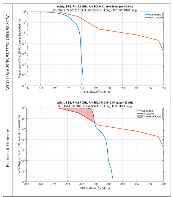
Figure 17 – Comparison of STEAM-1 (ID 121520025) EPFD  $\checkmark$  at 12.7 GHz with 0.45 m GSO ES for WCG and for Fuchsstadt, Germany (50.118°N. 9.924°E) with GSO Satellite at 17.6°E
