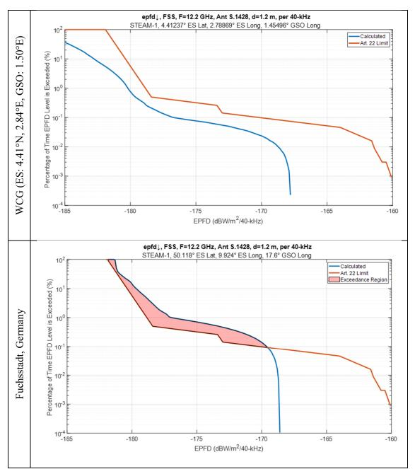
Figure 5 - Comparison of STEAM-1 EPFD↓ at 12.2 GHz with 1.2 m GSO ES for WCG and for Fuchsstadt, Germany (50.118°N. 9.924°E) with GSO Satellite at 17.6°E
