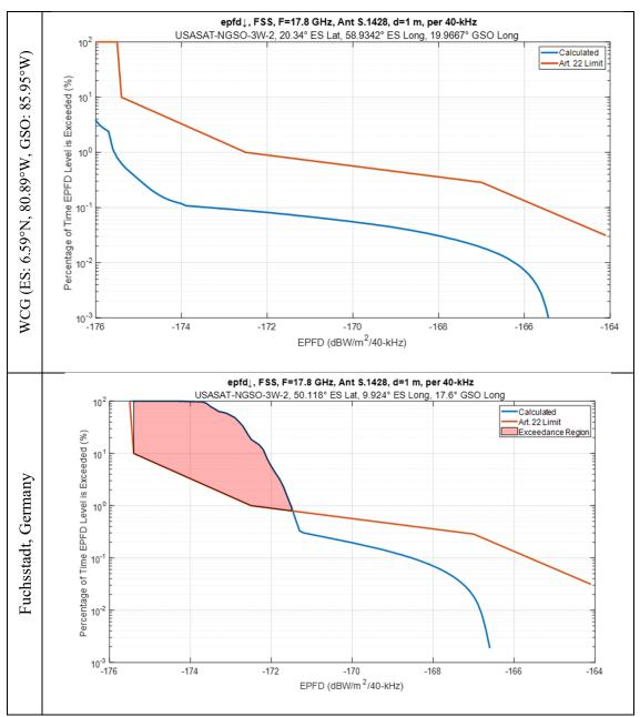
Figure 14 – Comparison of USASAT-NGSO-3W-2 EPFD  $\downarrow$  in 17.8 – 18.6 GHz Band with 1-m GSO ES for WCG and for Fuchsstadt, Germany (50.118°N. 9.924°E) with GSO Satellite at 17.6°E
