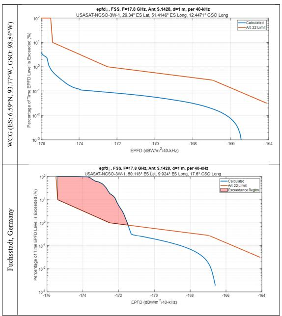
Figure 13 – Comparison of USASAT-NGSO-3W-1 EPFD $\downarrow$  in 17.8 – 18.6 GHz Band with 1-m GSO ES for WCG and for Fuchsstadt, Germany (50.118°N. 9.924°E) with GSO Satellite at 17.6°E
