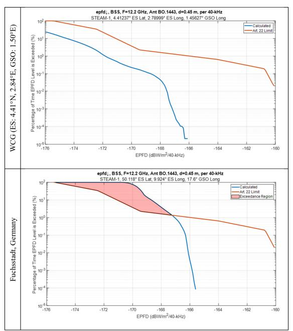
Figure 6 - Comparison of STEAM-1 EPFD↓ at 12.2 GHz with 0.45 cm GSO ES for WCG and for Fuchsstadt, Germany (50.118°N. 9.924°E) with GSO Satellite at 17.6°E
