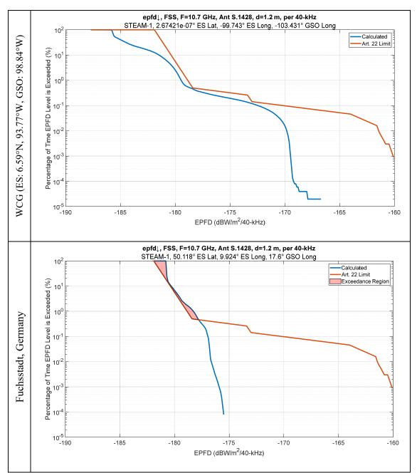
Figure 16 – Comparison of STEAM-1 (ID 121520025) EPFD  $\checkmark$  at 10.7 GHz with 1.2 m GSO ES for WCG and for Fuchsstadt, Germany (50.118°N. 9.924°E) with GSO Satellite at 17.6°E
